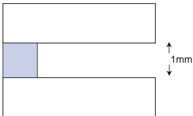
(a) Support structure with spacer wedged between the electrodes.
