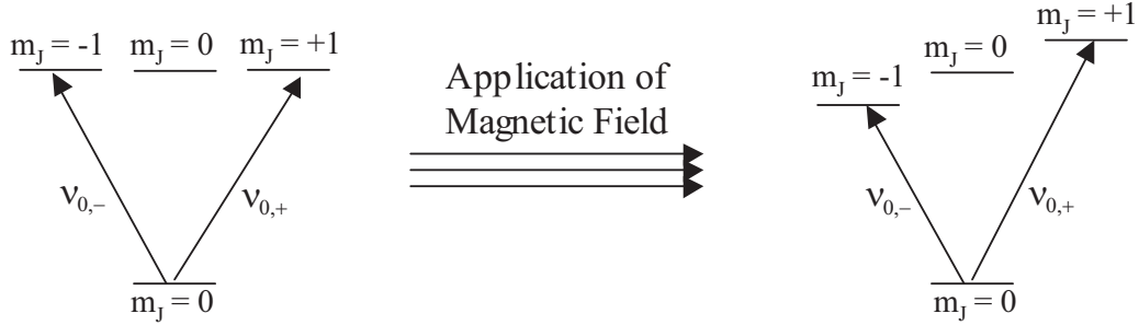
Figure 3.2: Before application of the magnetic field, \nu_{0,+} = \nu_{0,-} . After the magnetic field is turned on, \nu_{0,+} \neq \nu_{0,-} . This shifts the \sigma_+ resonant frequencies to higher values and the \sigma_- resonant frequencies to lower values.
